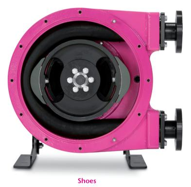
Fixed shoes move across the surface of the hose during compression. Typically this technology is preferred for higher operating pressures (up to 15 bar).
