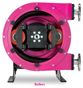
Rollers mounted on bearings compress the surface of the hose during rotation. This design generates less friction and mechanical stress on the hose and it can support pressures of up to 8 bar.
